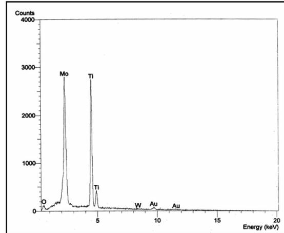
**Fig. 4.** EDS chemical analysis of dark areas in the treated layer sprayed with 100% Mo.
