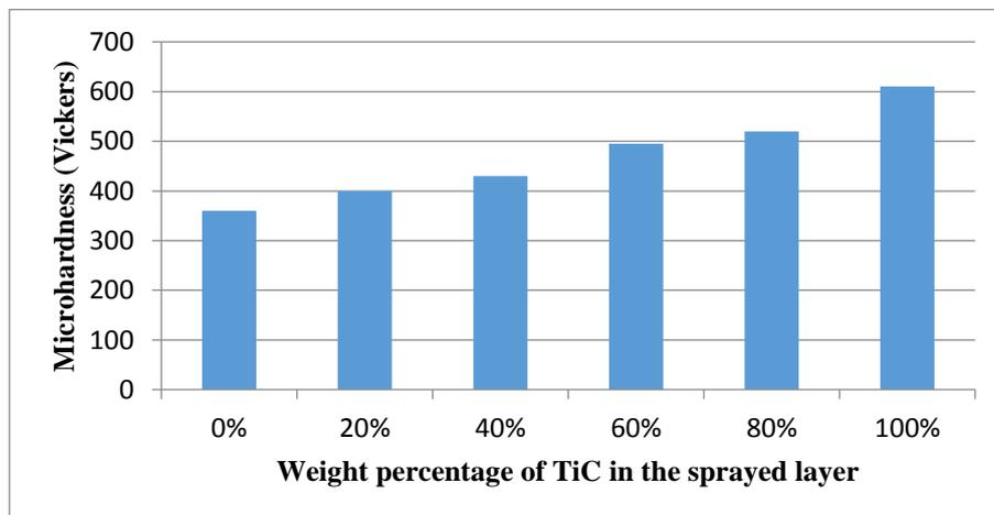
**Fig. 7.** Microhardness of treated layers with different ratios of Mo and TiC.
