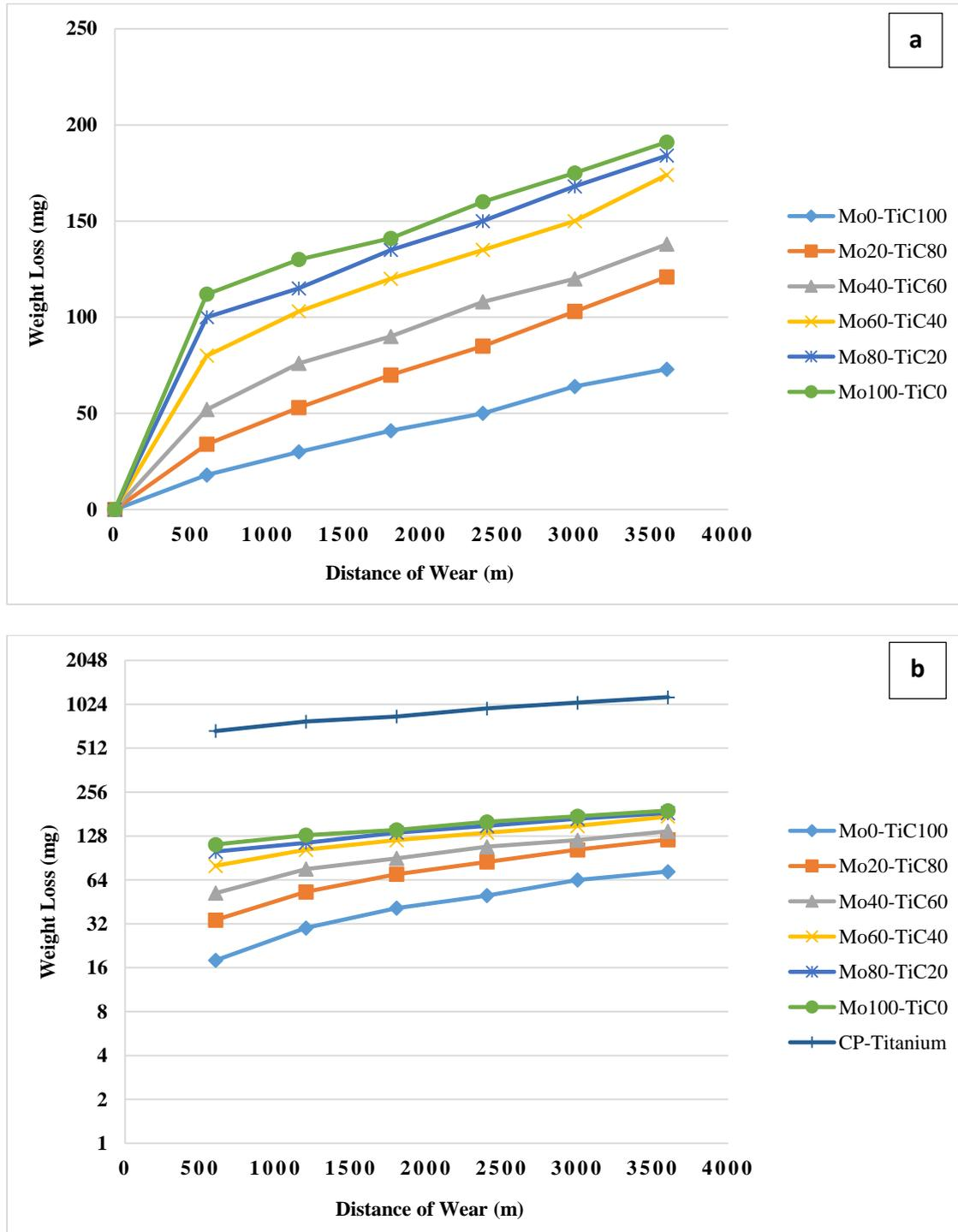
Fig. 8. Mass loss versus time of wear (a) coatings with different ratios of Mo and TiC, (b) different coatings in comparison with CP-Ti in logarithmic scale.
