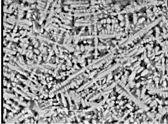
**Fig. 2.** The microstructure of the treated layer sprayed with 100% Mo.
