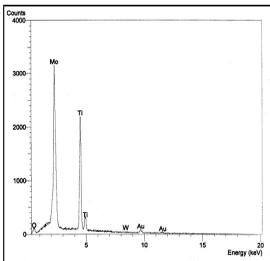
**Fig. 3.** EDS chemical analysis of bright areas in the treated layer sprayed with 100% Mo.
