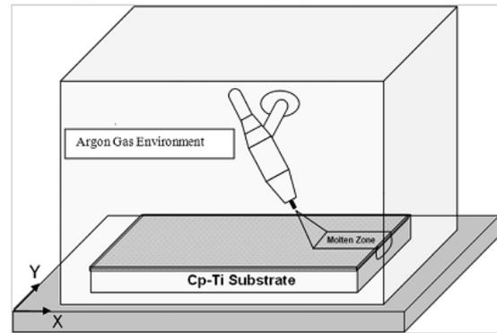
**Fig. 1. Schematic view of argon shielding box.**
