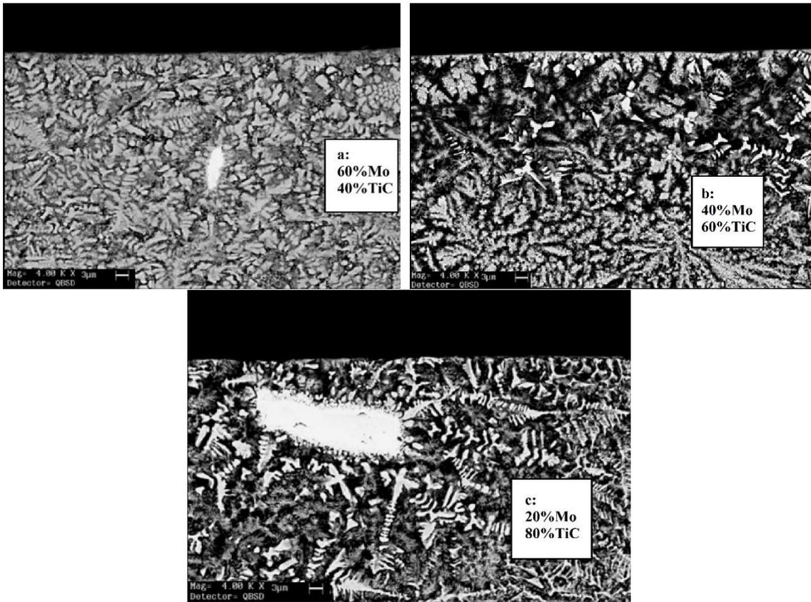
**Fig. 6.** The microstructures of treated layers with different ratios of Mo and TiC. (a) 60%Mo/40%TiC, (b) 40%Mo/60%TiC, (c) 20%Mo/80%TiC.
