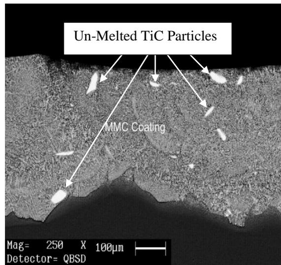
**Fig. 5.** Microstructure of treated layer sprayed with 80%Mo and 20%TiC.
