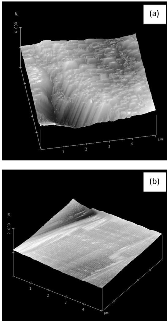
**Fig. 5.** AFM of titanium surface before and after oxidation. a) as-oxidized sample and b) grounded sample before oxidation
