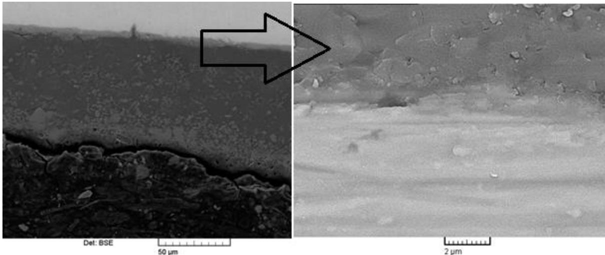
**Fig. 6. The glass ceramic appeared dense and well bonded to the substrate that was oxidized in 750°C for 30 min.**
