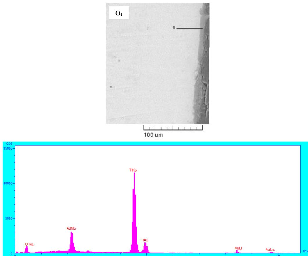
Fig. 4. SEM and EDS of O<sub>1</sub>, that heat treated at 750°C and 30 min.
