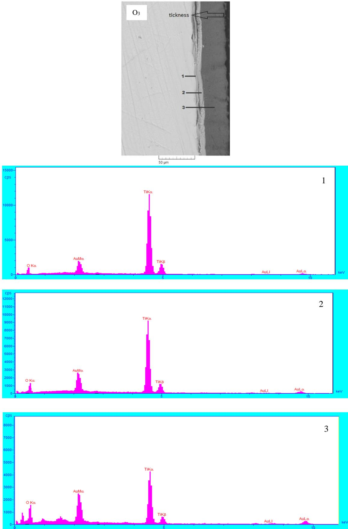
Fig. 2. SEM and EDS of O<sub>3</sub>, that heat treated at 750°C and 90 min.
