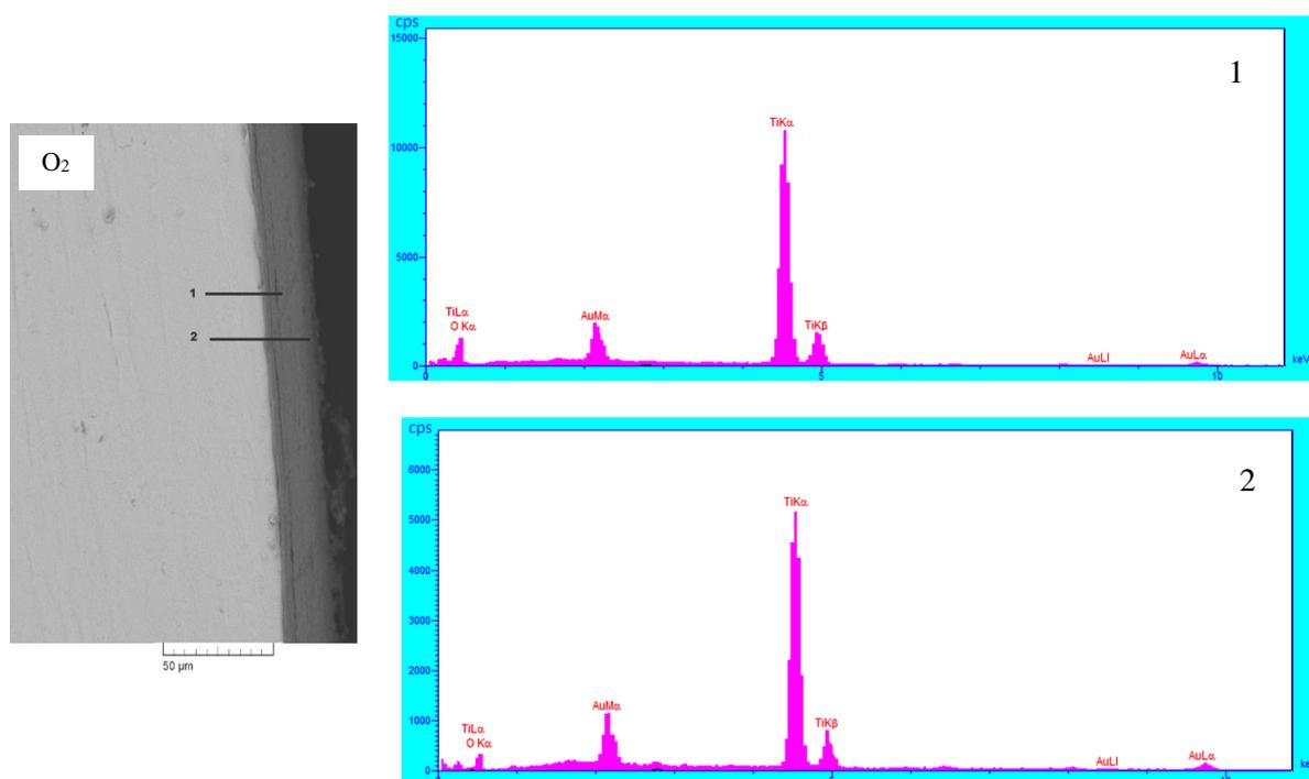
Fig. 3. SEM and EDS of O<sub>2</sub>, that heat treated at 750°C and 60 min.
