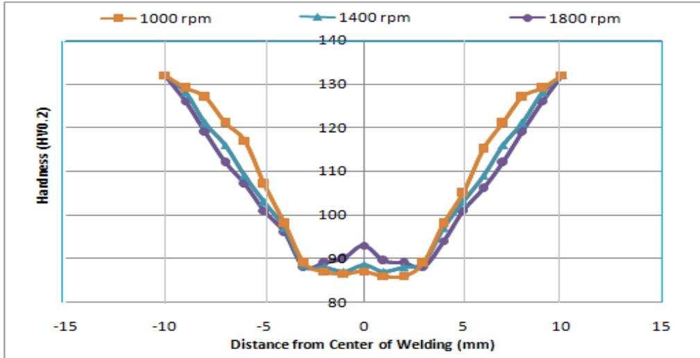
Fig. 11. The hardness distribution in various rotational speeds at flooding mode with travel speed of 80 RPM.
