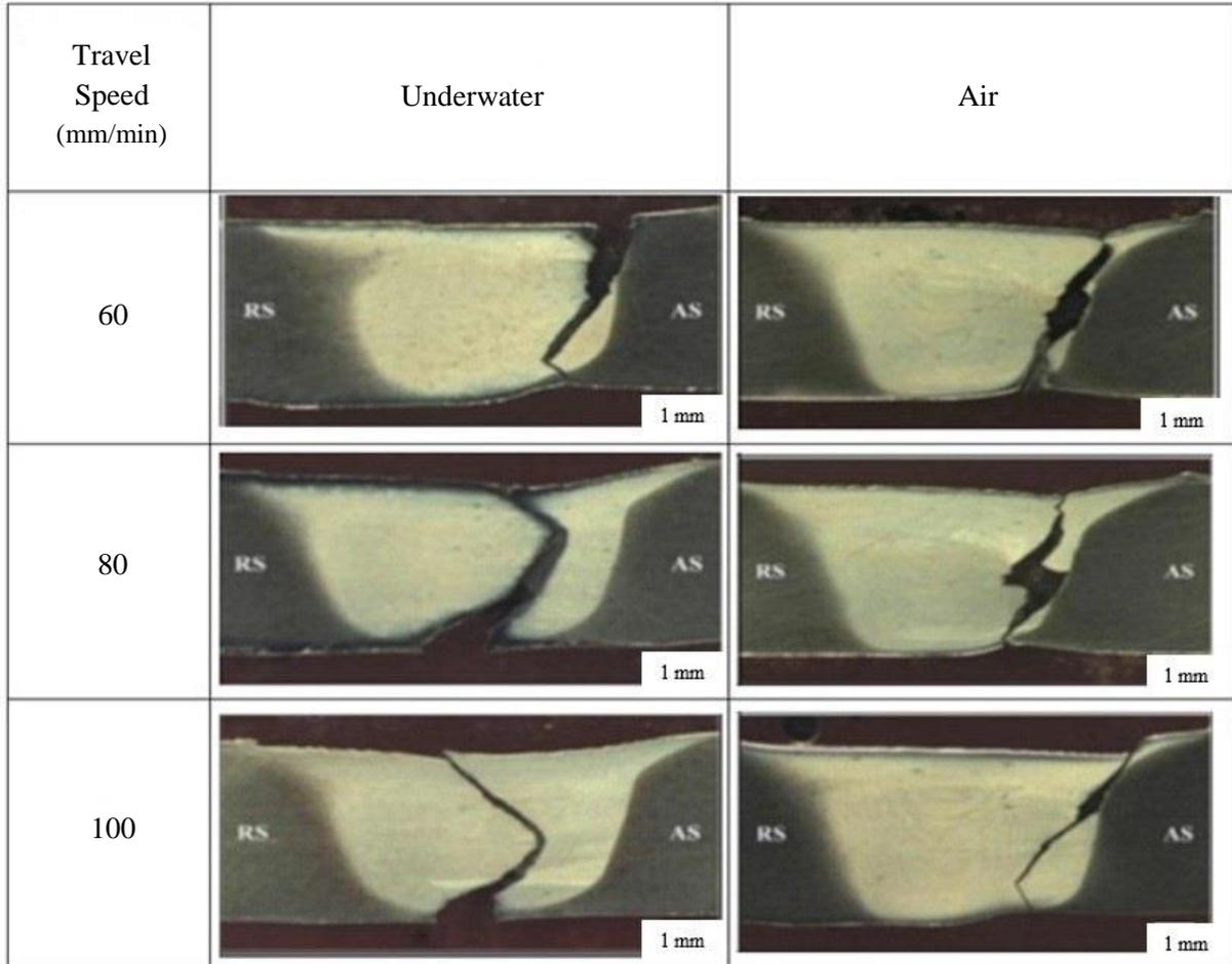
Fig. 7. The fracture zone of tensile samples in the different travel speeds at rotation speed of 1000 RPM.
