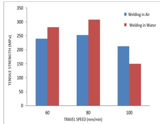
Fig. 6. The effect of forward speed on the tensile strength at rotational speed of 1000 RPM.
