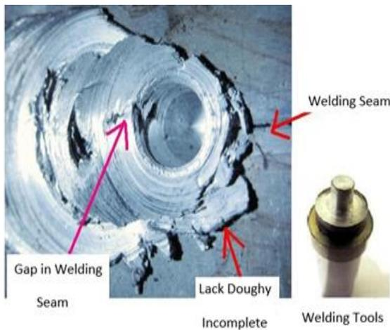
Fig. 9. Filings in the low rotational speed at flooding mode, welding by 500 RPM at air mode.
