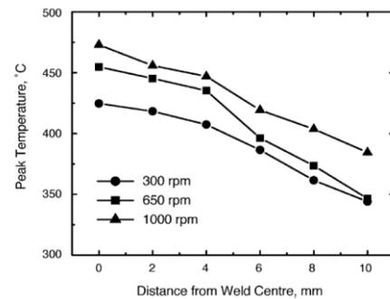
Fig. 1. The effect of the rotational speed on the maximum temperature [16].
