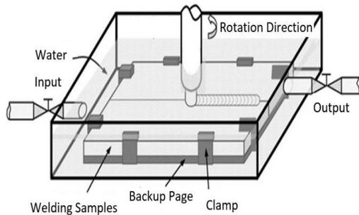
**Fig. 2. Schematic picture of underwater friction stir welding process.**
