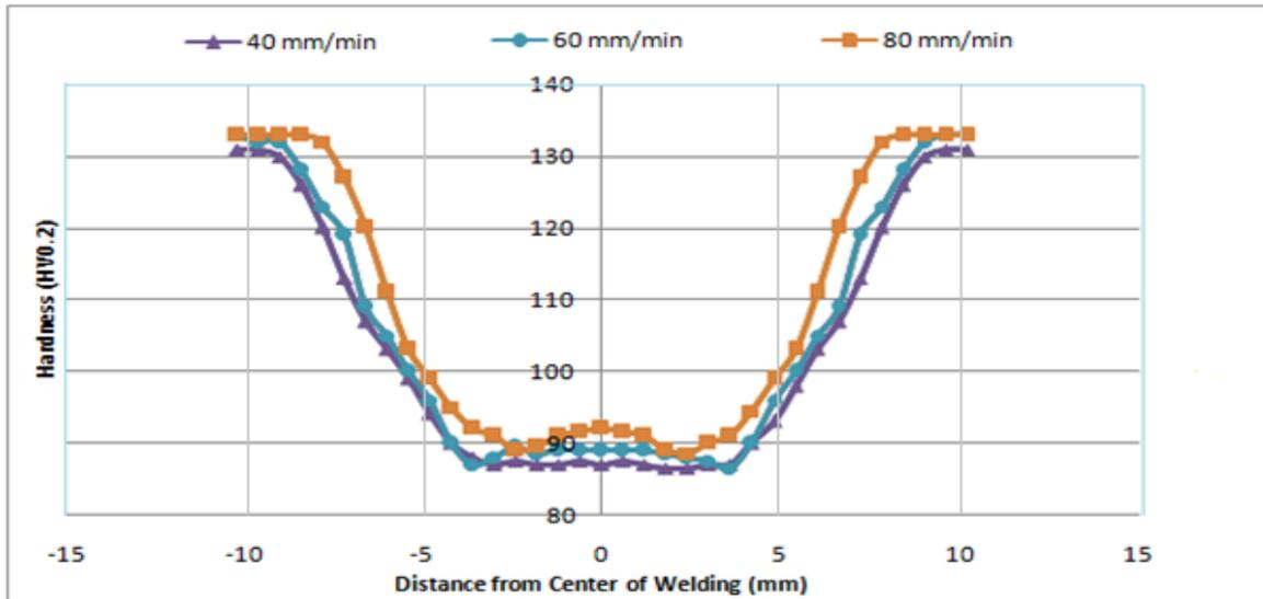
Fig. 8. The hardness distribution in the different travel speeds in underwater under 1000 RPM.
