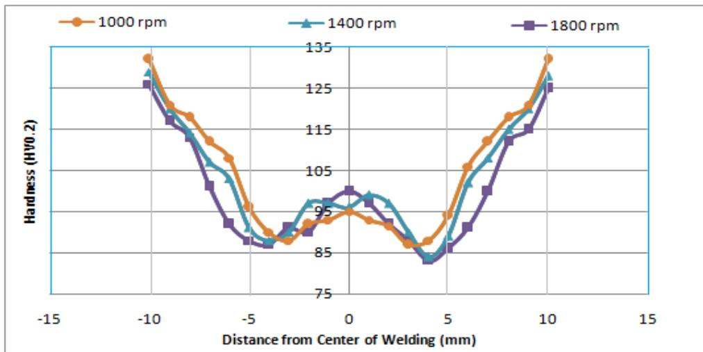
Fig. 12. The hardness distribution in various rotational speeds at normal mode with travel speed of 80 RPM.
