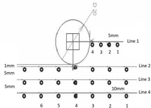
**Fig. 3. The temperature measurement sites on the piece and shoulder position of the tool.**
