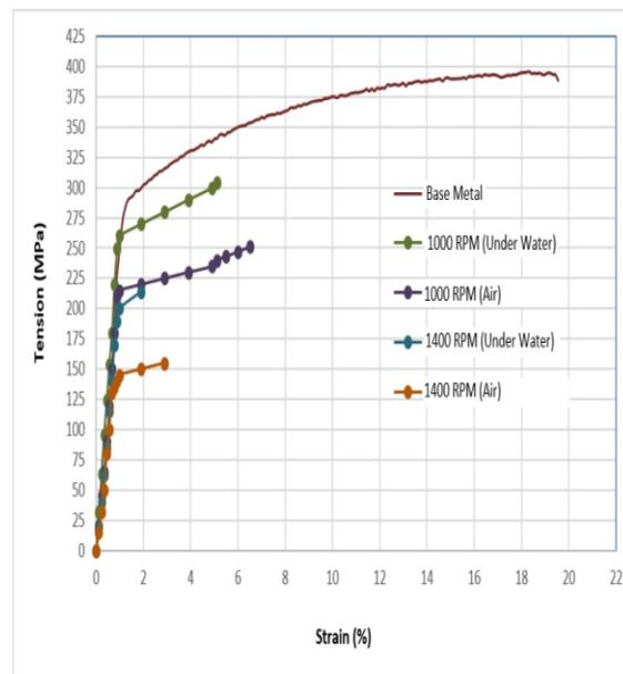
Fig. 10. The stress-strain curve at two different rotational speeds with travel speed of 80 mm per minute.
