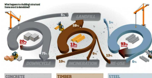
Fig. 2. Example of end-of-life scenarios for concrete, timber, and steel from the buildings [16].
