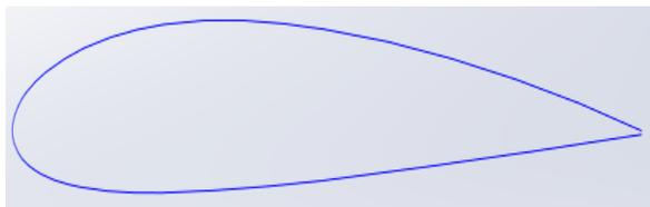
Fig. 2. Designed NACA2412 airfoil-section in SOLIDWORKS.
