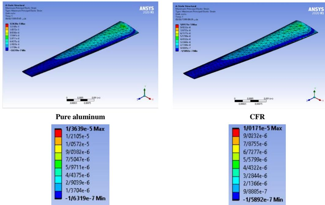
Fig. 8. Maximum principle elastic strain distribution of pure aluminum and CFR wing (Run by ANSYS Static Structural).
