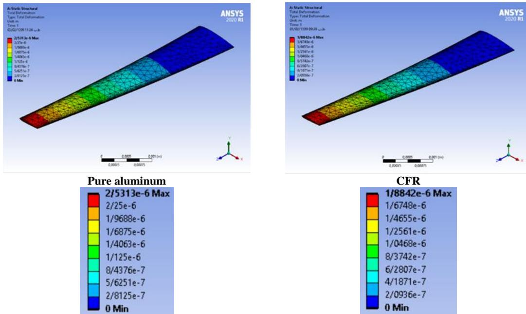
**Fig. 5. Total deformation distribution of pure aluminum and CFR wing (Run by ANSYS Static Structural)**
