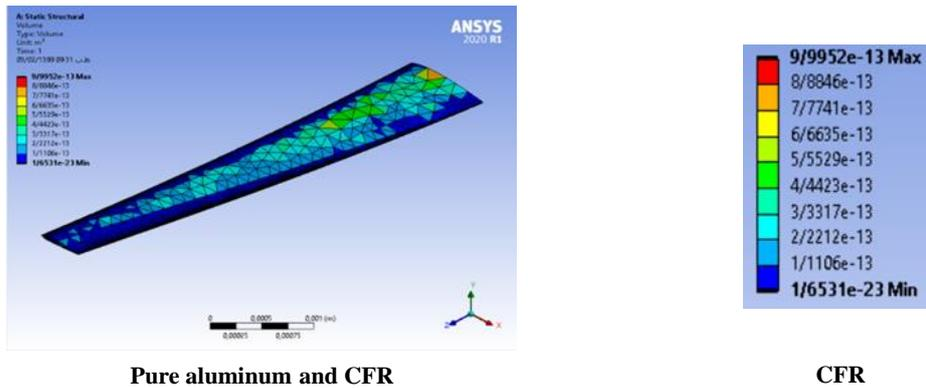
Fig. 11. Volume distribution of pure aluminum and CFR wing (Run by ANSYS Static Structural).
