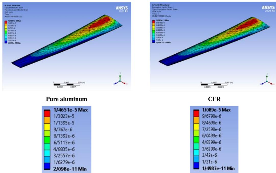
Fig. 7. Equivalent elastic strain distribution of pure aluminum and CFR wing (Run by ANSYS Static Structural)
