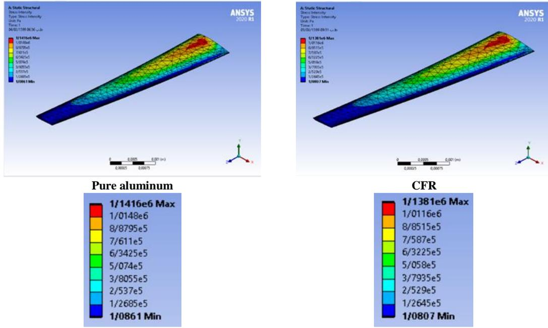
Fig. 10. Stress intensity distribution of pure aluminum and CFR win (Run by ANSYS Static Structural).
