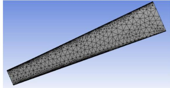
**Fig. 4. Meshed wing (Meshed by ANSYS Static Structure).**
