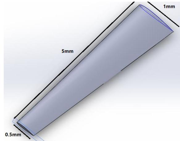
Fig. 3. Side view of a designed wing with dimensional isometric projection.
