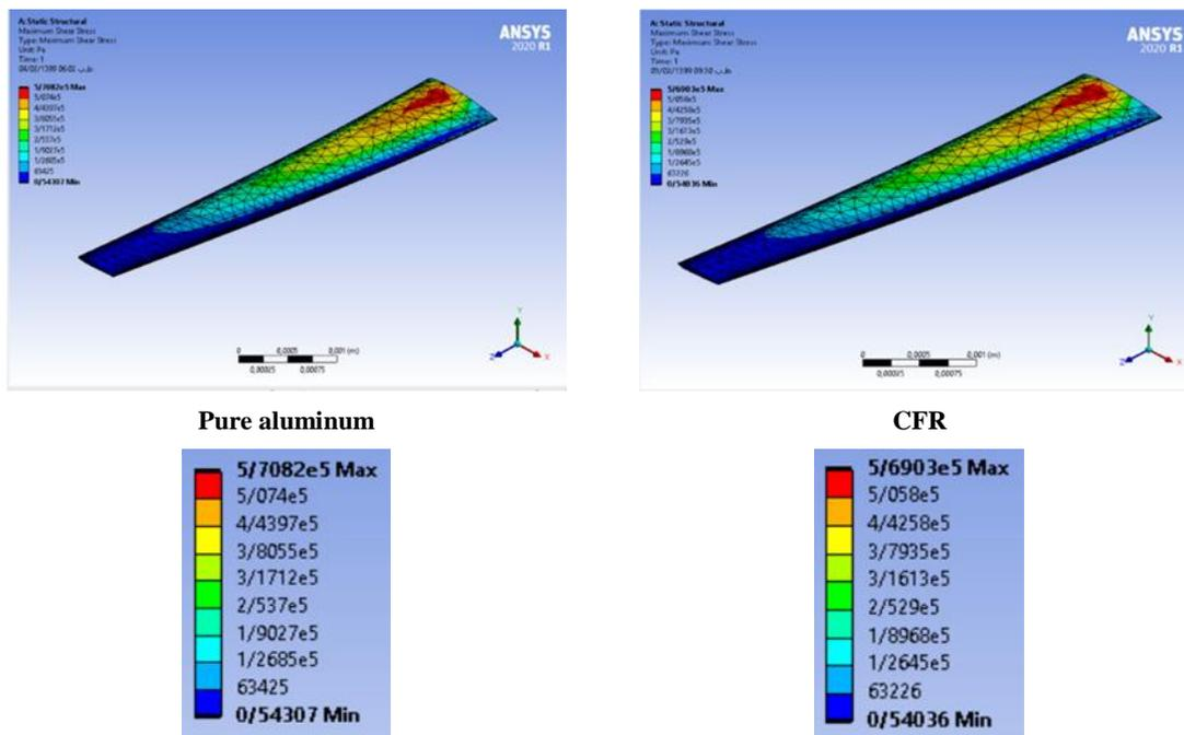
Fig. 9. Maximum shear stress distribution of pure aluminum and CFR wing (Run by ANSYS static Structural).
