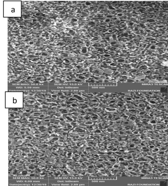
**Fig. 5.** FESEM microstructure of samples a-C1 and b-C2.
