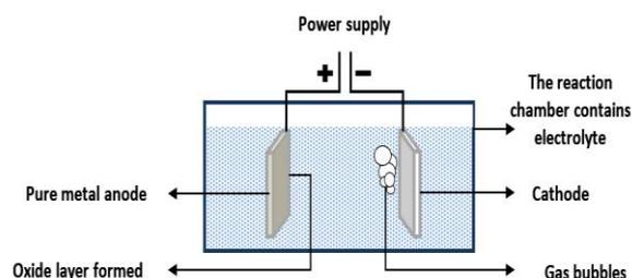
Fig. 1. Anodic oxidation process and its equipment [8].
