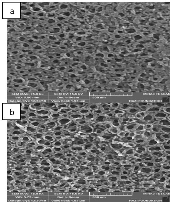
**Fig. 4.** FESEM microstructure of samples a-B1 and b-B2.
