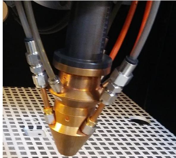
Fig. 4. Coaxial nozzle.
