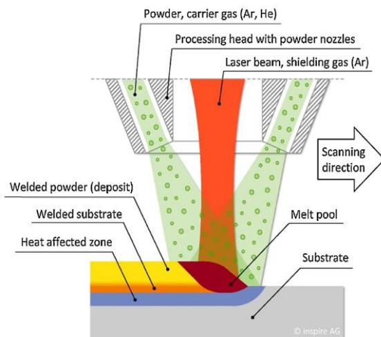
Fig. 3. A cross section of a coaxial LMD nozzle [10].
