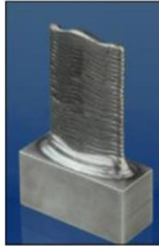
**Fig. 9. LMD process for blade building [56].**
