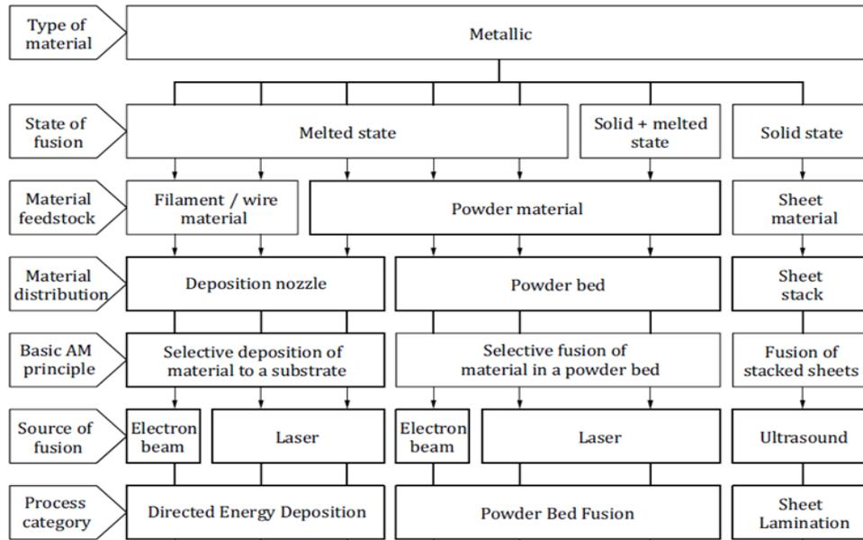
Fig. 1. Overview of single-step AM processing principles for metallic materials [4].
