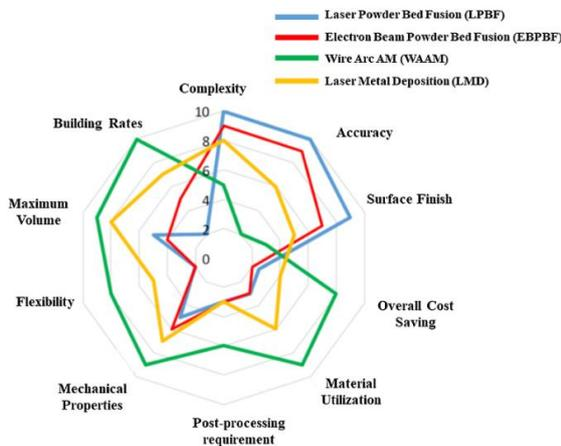
Fig. 2. Comparison framework among different metal AM technologies used in the aerospace industry [5].
