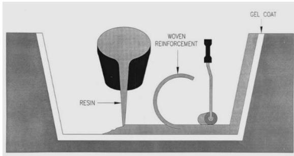
**Fig. 3. Hand lay-up method.**
