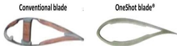
Fig. 2. Conventional blade vs One Shot blade technology
