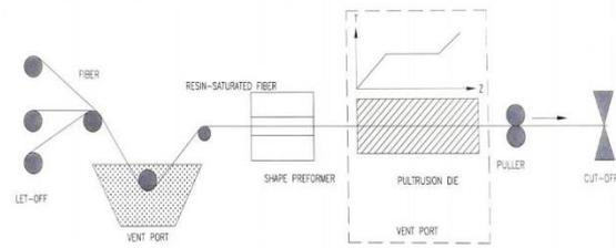
**Fig. 5. Pultrusion process.**
